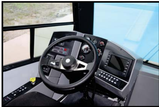
Ergonomically designed operator's platform with digital display and diagnostics.
