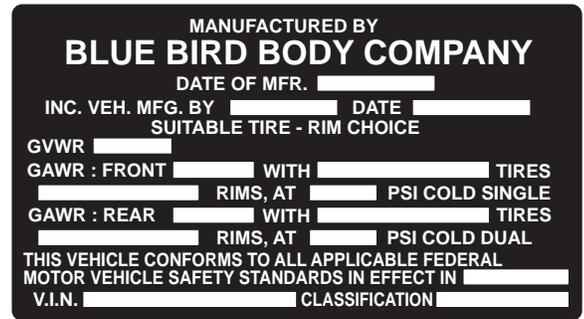
The **Body Serial and Service Number Plate** is located on the front upper inner panel above the windshield. Refer to the data on this plate for registration purposes or for replacement part information.
