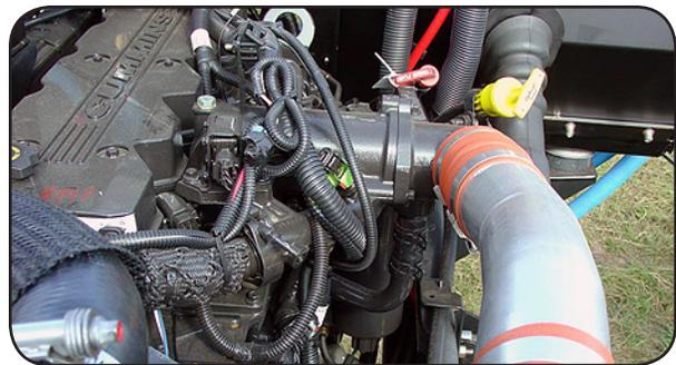
**4** Install charge air temperature switch 0115376 into the threaded fitting of the CAC tube, using Teflon pipe sealant tape.
