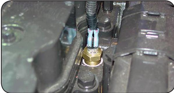
**6** Install the wiring for the new circuit. All wires added must be enclosed in .25" wire loom 1510775. Apply Glyptol to all the spade terminal connections made in the following steps:
