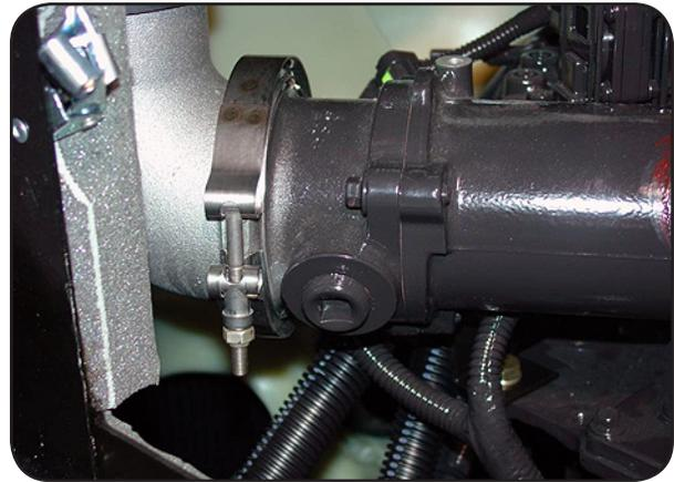
**3** Install the provided fittings in the charged air cooler intake adapter:
