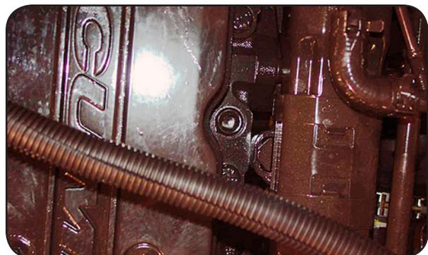
5.2 Remove and discard the plug. Install coolant temperature switch 0115375, using Teflon pipe sealant tape.
