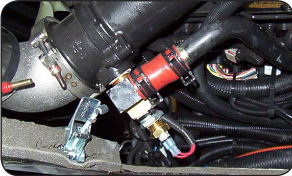
**4** Install coolant temperature switch 0115375:
