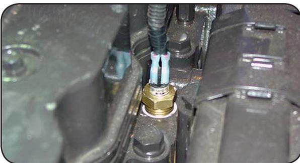
**5** Install the wiring for the new circuit. All wires added must be enclosed in .25" wire loom 1510775. Apply Glyptol to all the spade terminal connections made in the following steps:
