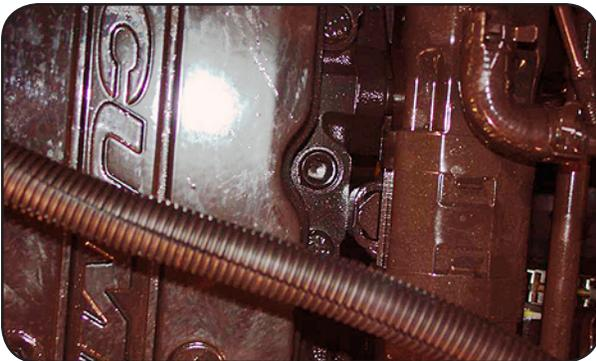
4.2 Remove and discard the plug. Install coolant temperature switch 0115375, using Teflon pipe sealant tape.
