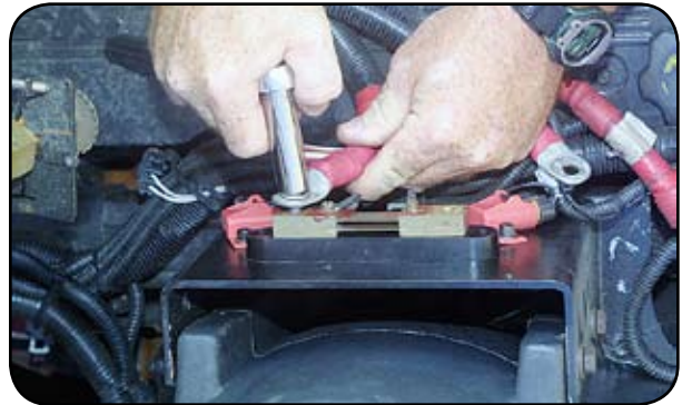
2 Small Signal Lead Screws Torque: 25-30 in lb.
