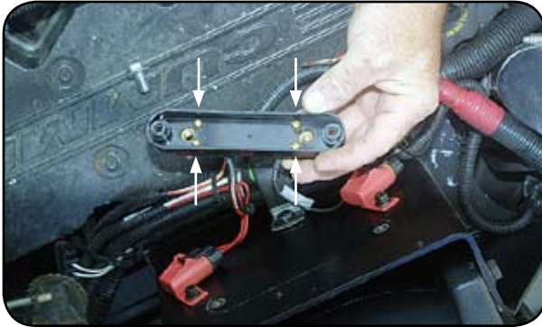
4 Shunt Base Screws Remove in order to discard existing plastic base. Use red Loctite upon re-installation.
