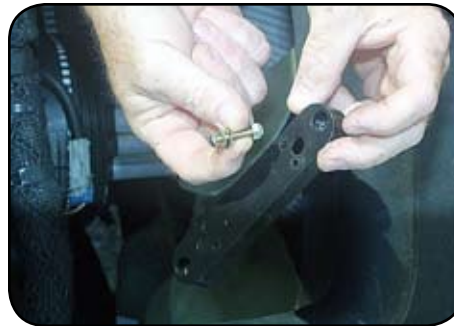
New Base Will be through-bolted to air cleaner bracket.
