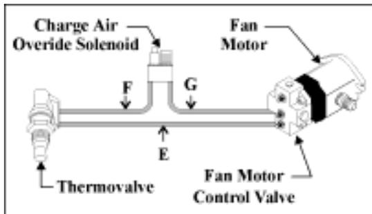
Figure 7—Pilot Control System Ports
