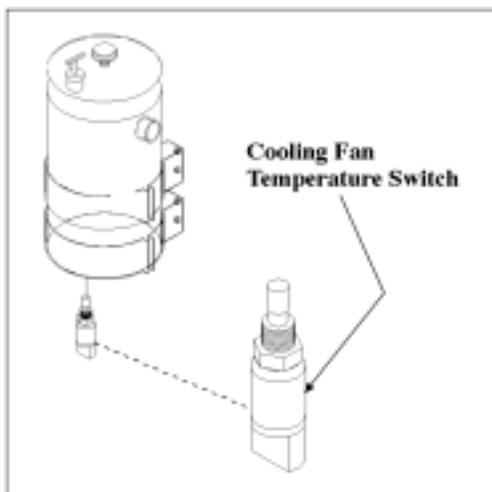
Figure 12—Cooling Fan Temperature Switch
