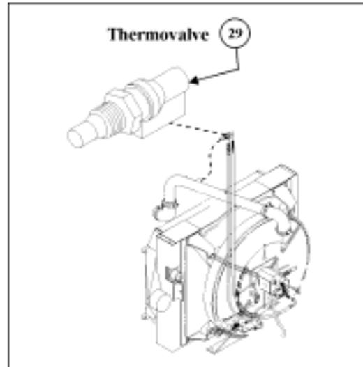
Figure 9—Engine Coolant Thermo-valve
