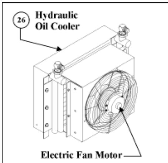
Figure 8—Hydraulic Oil Cooler
