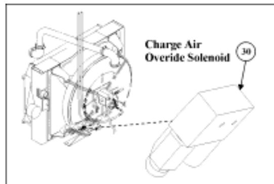
Figure 10—Charge Air Override Solenoid/Relief Valve
