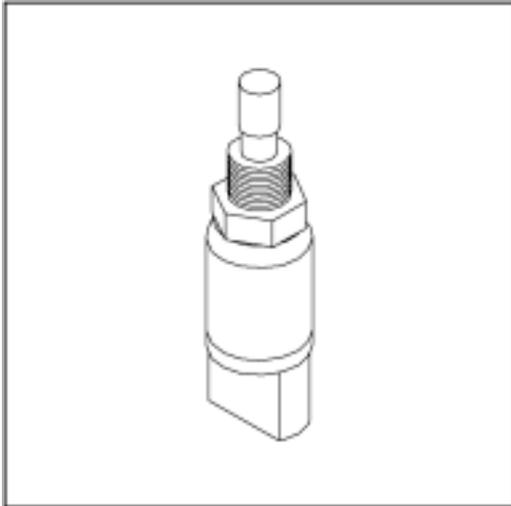
Figure 11—Charge Air Temperature Sensor
