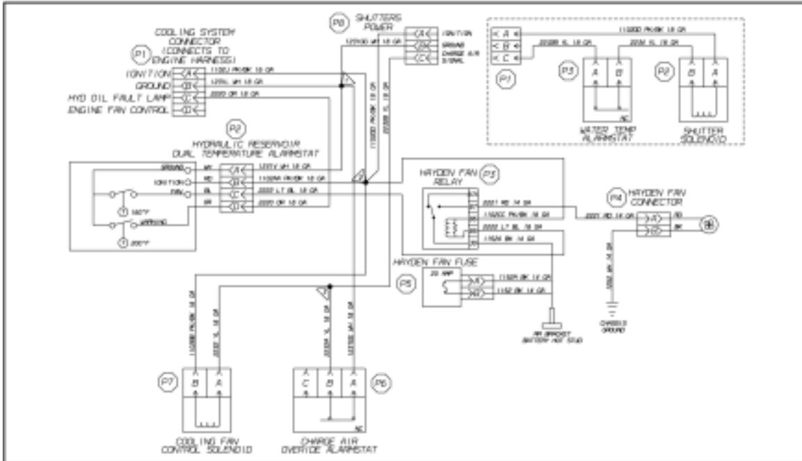
**Schematic 1—Hayden Hydraulic Oil Cooler Circuit**
