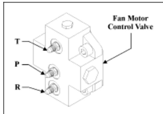
Figure 6—Fan Motor Control Valve
