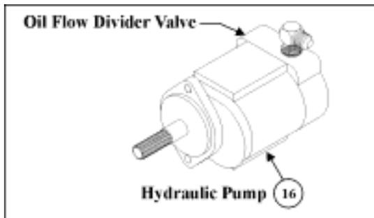
Figure 4—Oil Flow Divider Valve
