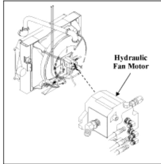
Figure 5—Hydraulic Fan Motor
