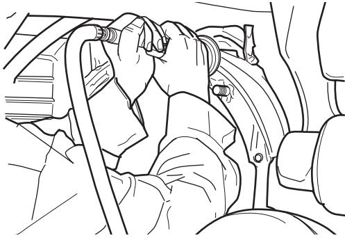
CLEANING HOUSING FACE WITH ROTARY TOOL AND SCOTCHBRITE™ PAD
