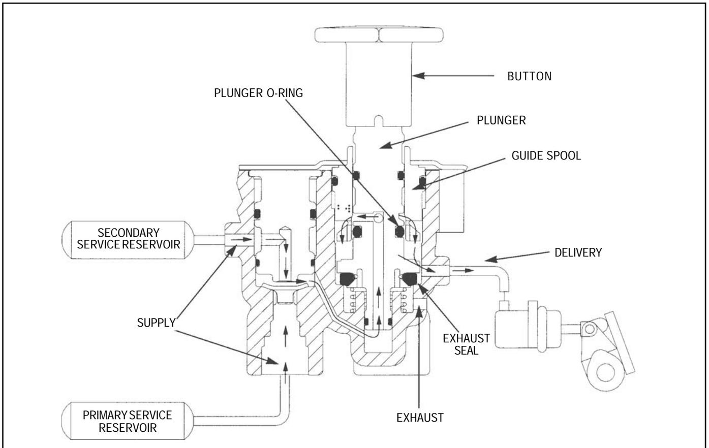
FIGURE 4 - SPRING BRAKES RELEASED (SECONDARY RESERVOIR SUPPLY)
