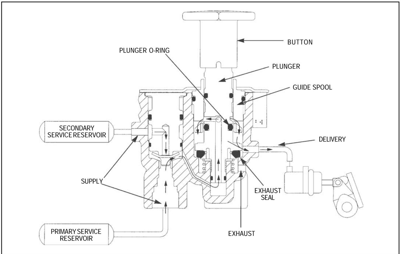
FIGURE 3 - SPRING BRAKES RELEASED (PRIMARY RESERVOIR SUPPLY)
