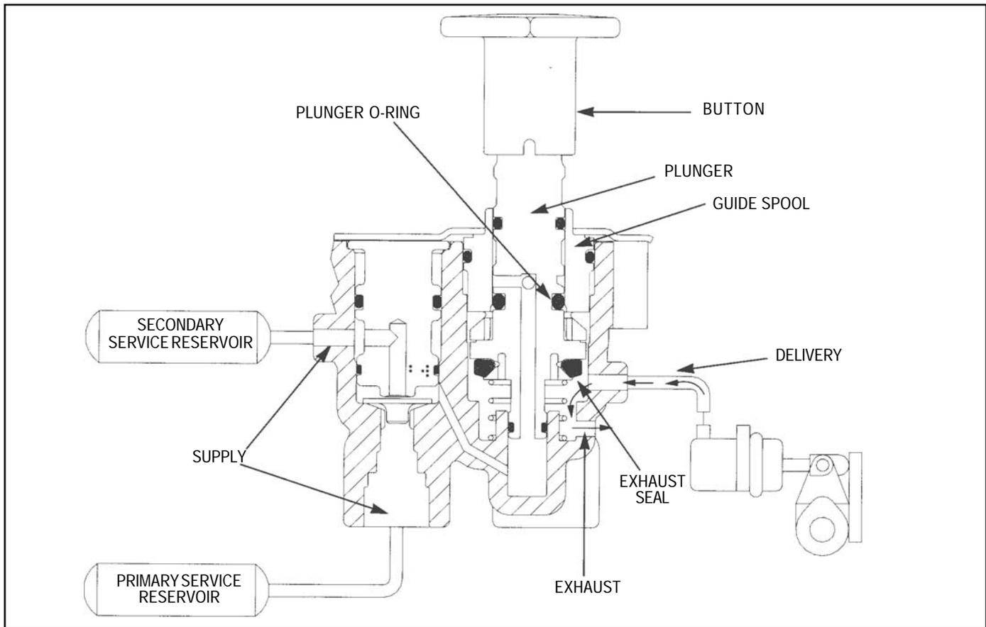
FIGURE 5 - PARKING BRAKES APPLIED
