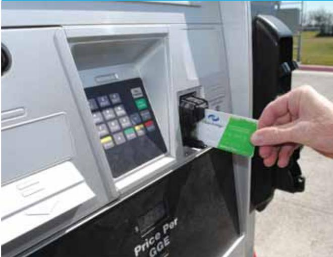
After securing the fill nozzle to the fueling connection receptacle, follow the instructions provided by the facility owner or operator to start the transfer of fuel. For facilities with an automatic dispenser, this may require running your credit card through a card reader.
