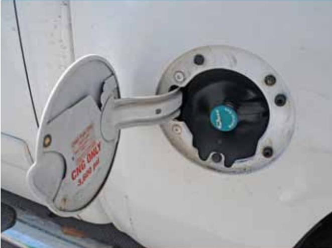
Remove the dust cap from the vehicle's fueling connection receptacle. The service pressure of the vehicle's CNG system—3,600 psi or 3,000 psi—is listed on the label next to the fueling connection receptacle.
