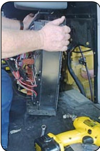
**6** Locate, inspect, and tighten the connections on the engine compartment side of the PDU panel as follows:
