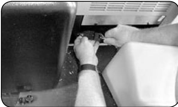
4.3 Remove two screws on each side of the PDU cover and remove the cover.
