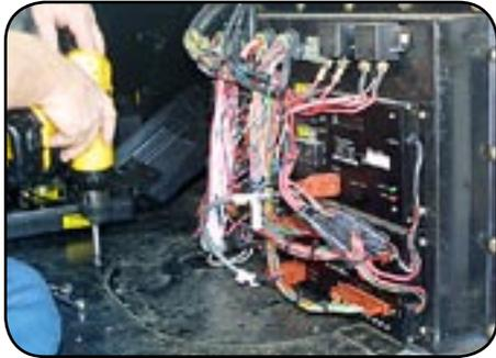
5.2 Remove the self-tapping bolts securing the PDU panel.
