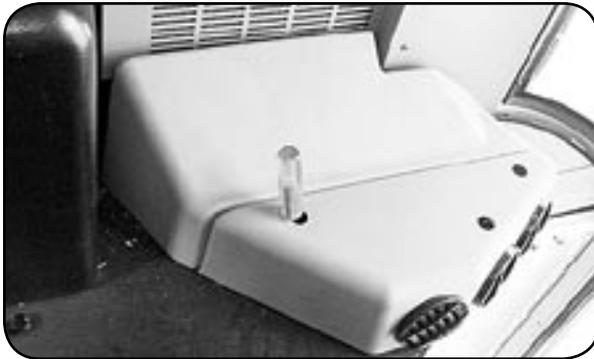
4.2 Slide the housing assembly rearward toward the stepwell. Unplug the blower motor harness at the left side of the assembly and remove the assembly.
