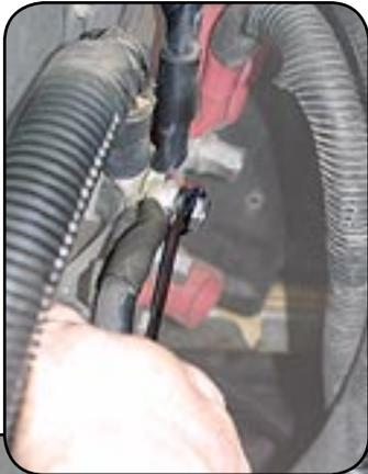
*Tighten all four connector stud nuts to 25 ft lbs. ...*
