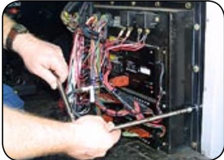
5.3 Carefully pull the right side of the PDU back just enough to allow access to the connectors, and power and ground studs on the engine side of the panel.
